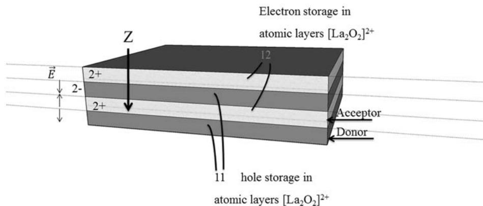
**Fig. (1).** Architecture of a typical high temperature superconductor made of stacks of atomic layers playing the role of Acceptors to storage photo-induced electrons and Donors to storage photo-induced holes.
